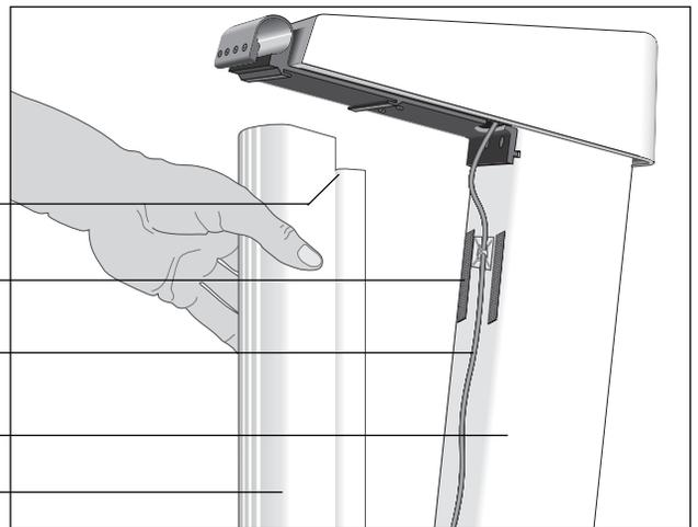
20. Attach the lift column trim by following these steps. While performing these steps, refer to Diagram 8 for further clarification.
