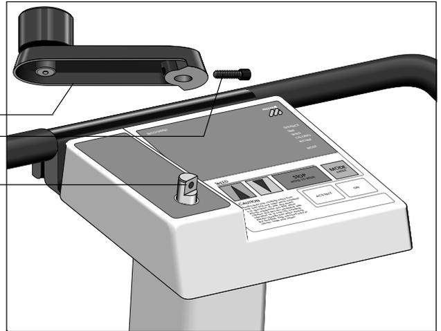
19. Install the incline crank handle (**M9.1 only**) onto the lift column shaft as shown in Diagram 7. Align the handle with the *flat* portion of the shaft end. Insert a screw (D) through the handle and crank shaft and tighten the screw securely with the hex key (G) provided. *Do not overtighten.*
