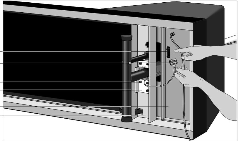
9. Route the ribbon cable as shown in Diagram 3, so that you have easy access to the receptacle on the motor chassis.
