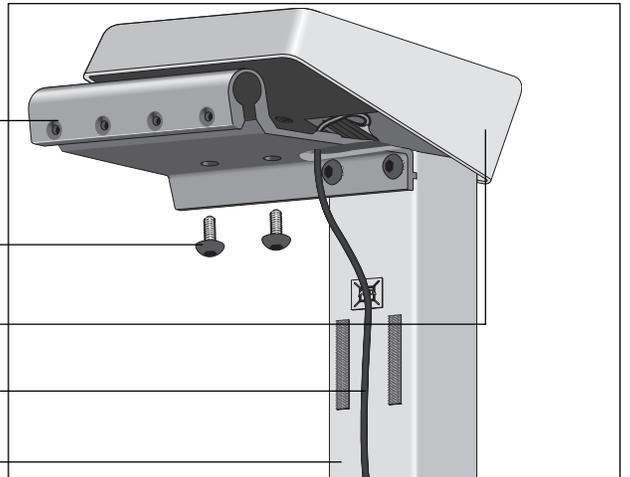
17. Align the electronic console mounting holes with the handrail clamp. Mount the electronic console onto the handrail clamp by inserting the two remaining handrail console screws (B). See Diagram 6. Insert the screws through the base of the handrail clamp and into the electronic console. Tighten the screws securely with the hex key (F) provided.
