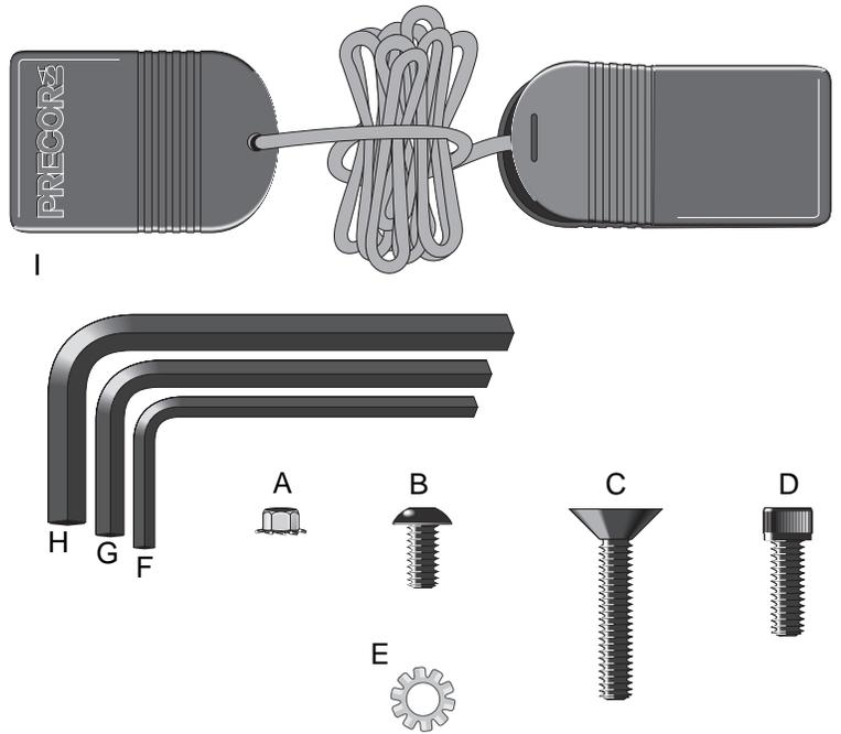
After unpacking the treadmill, open the hardware kit (refer to Diagram 1) and make sure that you have the following items:
