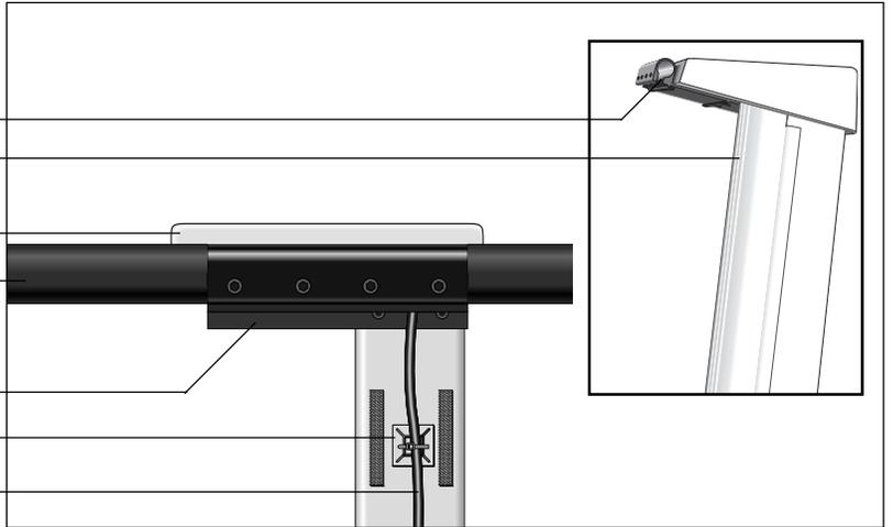
21. Insert the upper end of a handrail into the upper handrail clamp until the black foam wrap just touches the clamp. See Diagram 9. Set the base of the handrail on the floor. Repeat this step for the other handrail.
