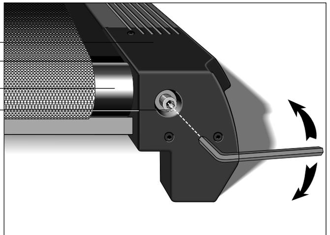
2. Standing behind the treadmill, use the rear belt adjustment bolts (each one at opposite sides of the rear roller). See Diagrams 15 and 16. Simply turn each bolt *clockwise* 1/4 turn to adjust the tension of the belt.
