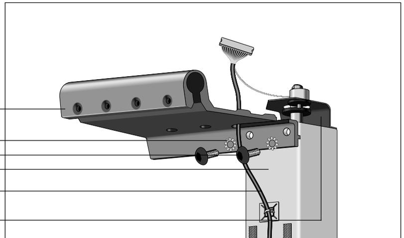
12. Place two external star washers (E) onto two of the upper handrail console screws (B) and align the upper handrail clamp with the mounting holes on the lift column. See Diagram 4.
