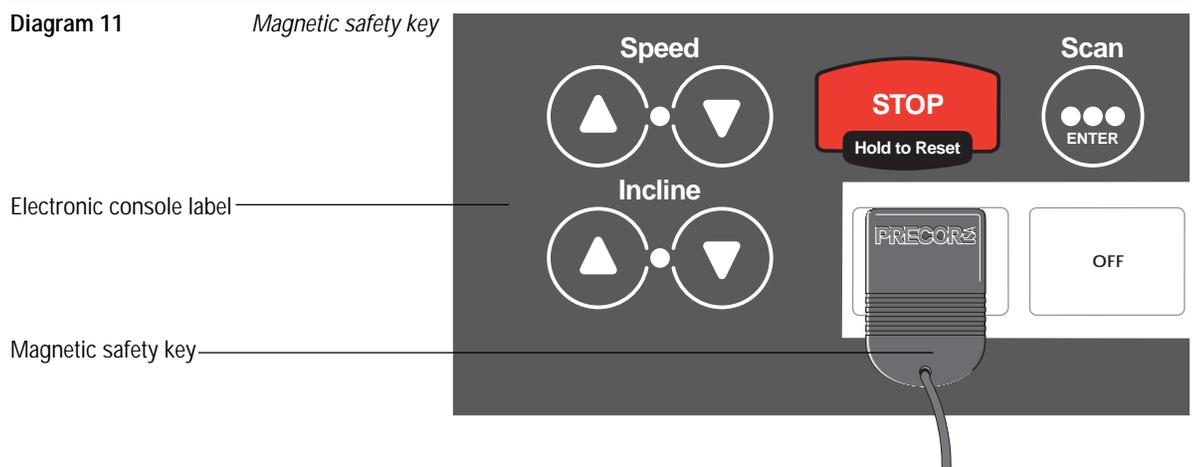
Before you can operate the treadmill, you must move the magnetic safety key to the ACTIVATE position on the electronic console. See Diagram 11. The treadmill will not turn ON unless the safety key is in this position.
