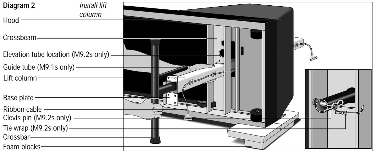
3. Pick up and rotate the lift column so that the crossbar is at a 90 degree angle to the base of the treadmill. The guide tube, **on the M9.1 only**, should align with the grommet hole in the crossbeam. Refer to Diagram 2. If necessary, remove the lower cable connector from inside the crossbar.
